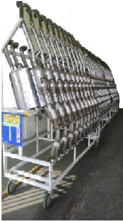
① Exhaust Pipe Trolley Corolla (Loads)
